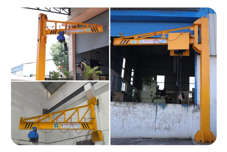
A **JIB Crane** Is A Type Of Overhead Lifting Device That Is Often Used In Smaller Work Areas For Repetitive Lifting Tasks. Jib Cranes Are Highly Adaptable And Can Be Paired With Overhead Bridge Cranes To Increase Production.
