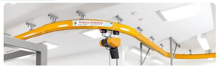
A **Monorail Cranes** Consist Of A Single Rail Or Track System Along Which The Hoist And Trolley Move. This Design Allows For Smooth And Precise Movement Of Loads, Optimizing Material Handling
