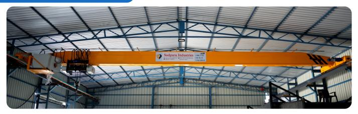
A **Single Girder EOT Crane** Is A Crane That Is Designed For Light And Medium Duty Material Handling. They Are Used For Short Period Work And Light Duty Weight. They Are Ideal For Facilities And Operations With Limited Floor And Overhead Space.
