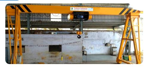
A **Goliath Crane** Is An Overhead Crane That Uses Legs To Support A Bridge, Trolley, And Hoist. The Legs Move On Wheels Or Rails Implanted In The Ground. Goliath Cranes Are Also Known As Goliath Cranes. They Are Mounted On Top Of A Structure That Extends Over An Object Or Workspace. The Structure Is Called A Goliath, Which Is Where The Crane Gets Its Name.
